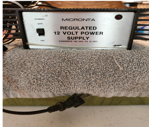
Micronta 22-120 Power Supply Regulated 13V @ 2.5 Amp
