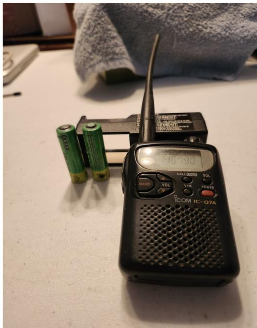
The very compact **Icom IC-Q7A** covers both the 2 Meter and 440 MHz amateur bands. It also provides exceptional triple conversion receive coverage from 30 to 1300 MHz (less cellular) in AM, FM-N and FM-W. Ten different tuning steps from 5 kHz to 100 kHz are supported along with six types of scanning. Advanced features include: 200 memories, CTCSS encode/decode, backlit LCD, RIT, Power Save and Lock. Output is 350 mW on 2 Meters and 300 mW on 440 MHz
