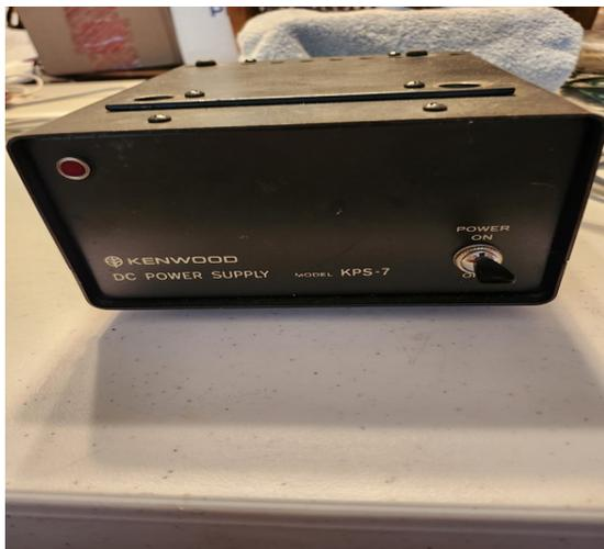
The **Kenwood KPS-7** power supply provides 13.8 VDC at 7 Amps intermittent (ICS), or 6 Amps at continuous load. Input is 120 VA. The [rear panel](#) has a heat sink, red and black binding posts and a removable 2 Amp fuse. 6 x 4 x 9 inches.
