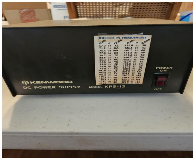
The **Kenwood KPS-12** power supply provides 13.8 VDC at 12 Amps intermittent (50% duty cycle) or 10 Amps continuous. Input is 120 VAC. The [rear panel](#) has red and black terminals. 7.785 x 4.785 x 9" 14.6 lbs.
