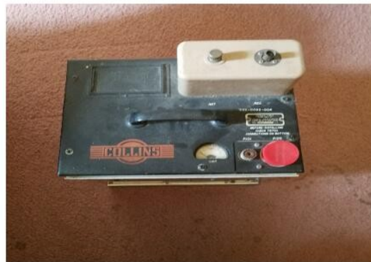
Remote Antenna Tuner Picture 2
